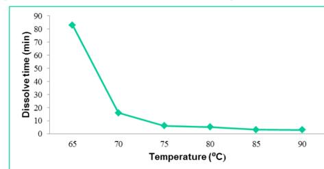
Figure 2 shows water sensitivity of biodegradable polymer. The film was dissolved at 65°C water in 83 minutes, while at 70°C water in 16 minutes. When the temperature increased up to 90°C, dissolved time decreased to 3 minutes.
