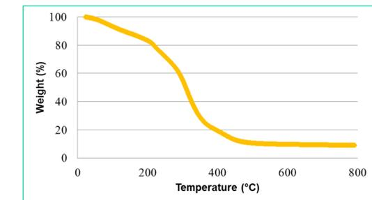
Figure 4 shows the TGA results generated on starch-based biodegradable polymer. The plot indicates the percent mass as a function of sample temperature for the polymer. Maximum weight change was observed between 200°C and 400°C. Beyond that point, weight change rate decreased. It was also determined that the biodegradable polymer leaved about 9 wt % of residue at 800°C in nitrogen atmosphere..
